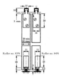
Aluminium top channels with nylon guides and aluminium bottom rails with nylon rollers for quiet, smooth operation of wood-framed glazed or flush, bi-passing cupboard or cabinet doors. Multiple tracks can be fitted.
