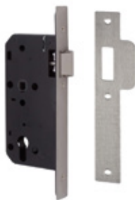
DDA 55mm backset 72mm C/C euro mortice nightlatch case only to BS EN 12209
