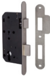
DDA 55mm backset 72mm c/c euro mortice sashlock case only to BS EN 12209
