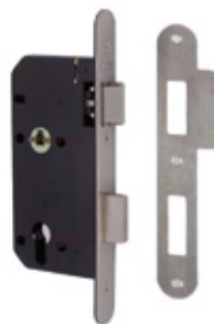
DDA 55mm backset 72mm C/C euro mortice escape lock case only to BS EN 12209
