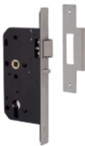
DDA 55mm backset 72mm C/C euro mortice deadlocking nightlatch case only to BS EN 12209 sq forend
